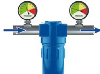
Resistance to pressure, otherwise known as Differential pressure (pre- and post equipment)
